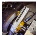
The pipe beveling machine is used for weld prep of tube and pipe end in pipe welding applications. Especially for heavy wall pipes the machining is fast and accurate. Pipe beveling and facing can be done in one operation with special tool holders. Operated by one worker the pipe beveling machine can be used in the workshop and on site with low weight due to aluminum construction. High speed beveling and facing with special tool bits provides economical manufacturing of pipes, tubes and headers.
